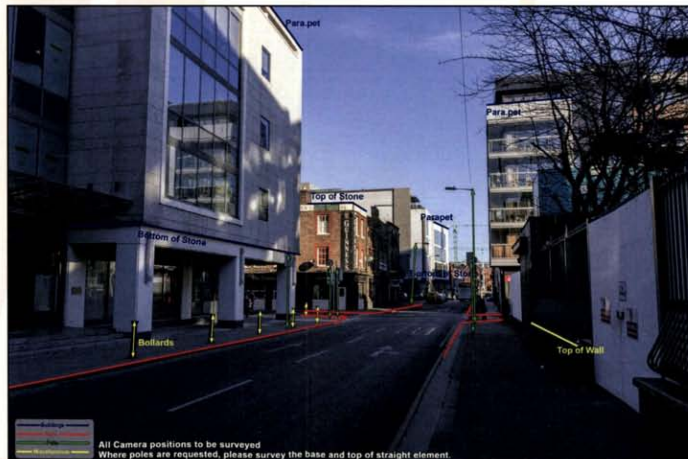
Fig.7: Fixed reference points marked for surveyour.
